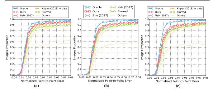
**Fig. 11** CED plots for the landmark localization experiment of Sect. 5.4. To avoid cluttering the plot, only the top 3 methods along with the oracle and the original blur performance are plotted. From left
