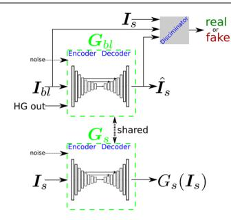
**Fig. 3** Schematic of our cGAN (Sect. 3.2). The training time cGAN is depicted in the left. 'HG out' signifies the additional label used as input, i.e. the output of the HG network, while the weight sharing of the
