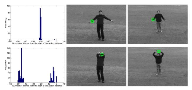
Fig. 6. Ensemble weighting example for the temporal case. Ensembles that are activated at a specific phase of the action receive a large weight (top row). Conversely, ensembles that are activated at more than one instances receive a smaller weight (bottom row).
