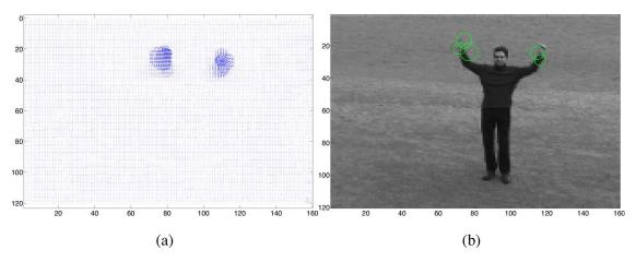
Fig. 3. (a) Estimated optical flow field for an instance of a handwaving action and (b) a subset of detected salient points.
