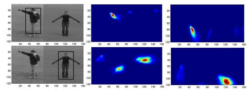
Fig. 14. Voting spaces for center and lower bound derived using the (a) boxing and (b) handwaving models, and rectangles fitted around the subjects using these voting spaces. Notice that each model favors votes belonging to the activity it was trained for.
