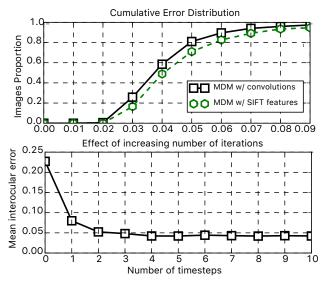
Figure 5: *Top*: Comparison between hand-crafted SIFT features vs. end-to-end CNN features tailored for face alignment. *Bottom*: Increasing the number of time-steps decreases the average error but stabilises after four iterations.
